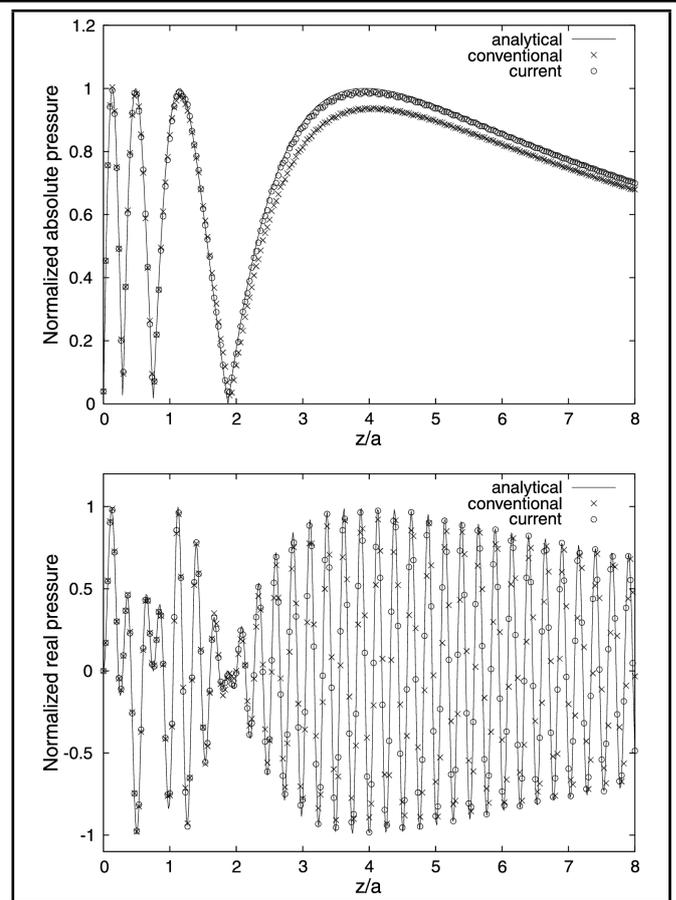
**Figure 10.** Comparison of the numerically and analytically obtained normalized pressures  $|\bar{p}|/(2\rho_f cv_n)$  and  $\bar{p}_r/(2\rho_f cv_n)$  along the axis of the piston as a function of  $z/a$  for  $ka = 8\pi$ .
