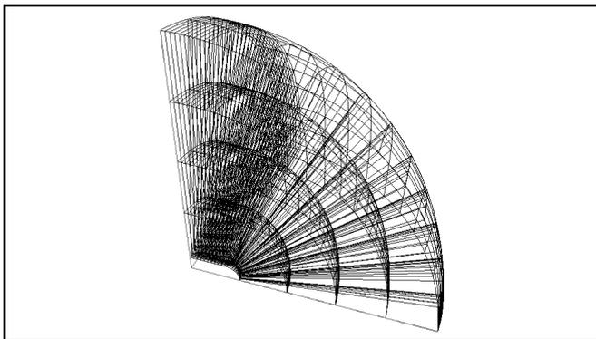
**Figure 9.** A typical mesh for the cylinder with hemispherical end caps problem; for clarity, fewer elements are shown in the radial direction than actually used.
