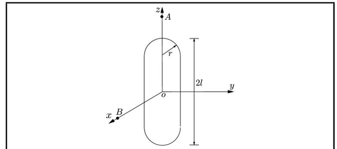
Figure 8. Pulsating cylinder with hemispherical end caps.
