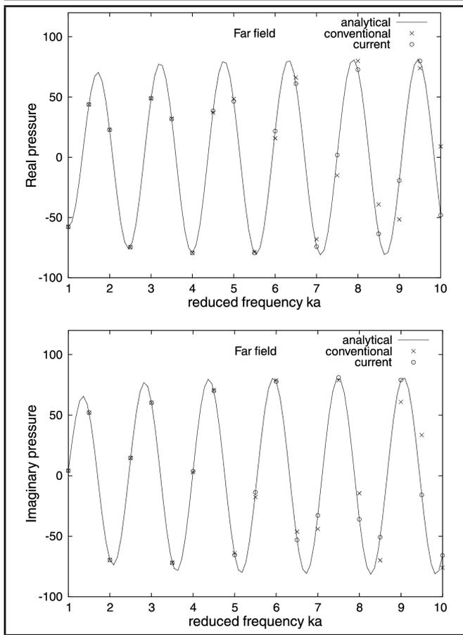
**Figure 2.** Comparison of the numerically and analytically obtained real and imaginary parts of the pressure at  $r = 50$  for various frequencies in the pulsating sphere problem.
